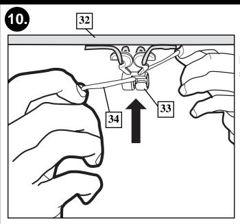
Insert net into bottom of clip as shown.
